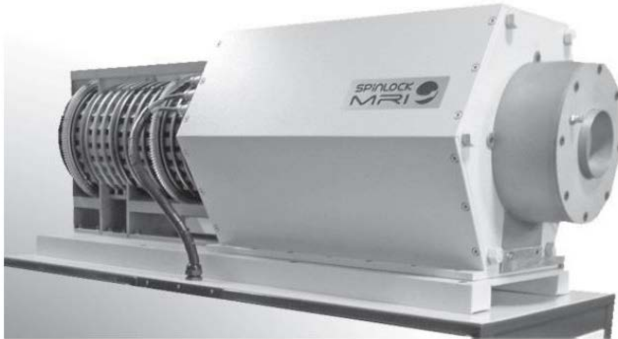
Figure 5. Halbach magnet for flow analysis with pre-polarizer magnet (Colnago et al., 2014).
